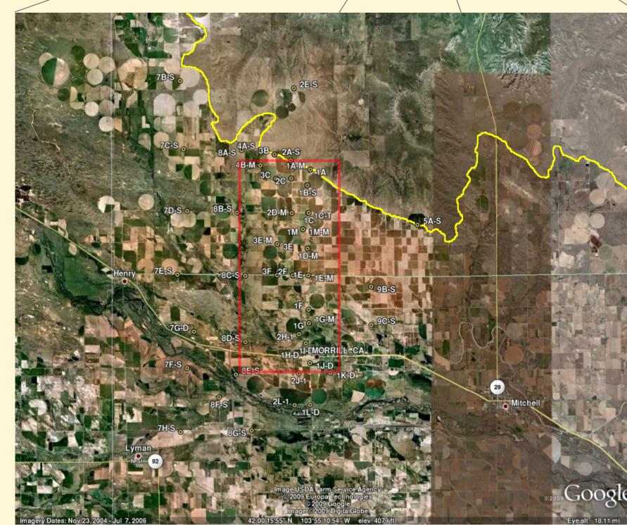
Dutch Flats, NE infiltration site and monitoring network. Gravity stations are located on existing well clusters, labelled in the detail map with yellow circles and names. Infiltration is controlled by a large, unlined irrigation canal at the north edge of the main network (shown in yellow). The regional hydraulic gradient across the network is to the south; following maps refer to the area boxed in red.
