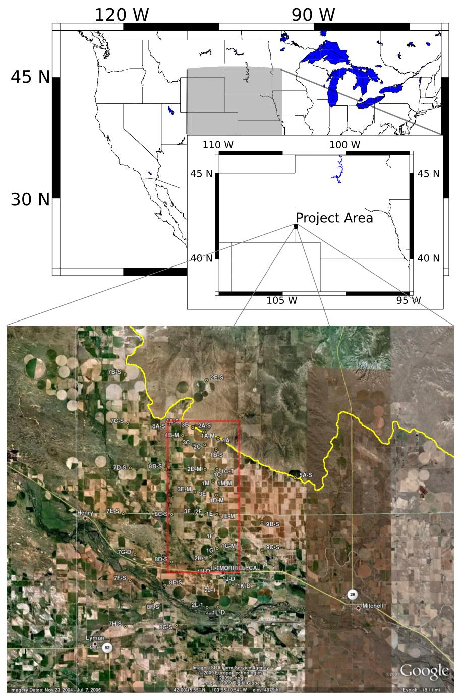
Dutch Flats, NE infiltration site and monitoring network. Gravity stations are located on existing well clusters, labelled in the detail map with yellow circles and names. Infiltration is controlled by a large, unlined irrigation canal at the north edge of the main network (shown in yellow). The regional hydraulic gradient across the network is to the south; following maps refer to the area boxed in
