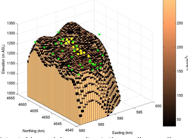
The gravity effect of the model is computed using a method of moments (Grant & West, 1965). Gravity effects from two models are differenced for comparison with the observed gravity changes at stations, as a function of assumed porosity.
